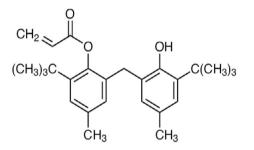
MBPA is a heat and light stabiliser and an antioxidant used in a wide range of adhesive, plastic, and elastomer materials. This substance is an effective alkyl radical scavenger, which property is especially useful in processes at high temperatures and in low oxygen environments, such as during the initial mixing of adhesives.<sup>52</sup>
